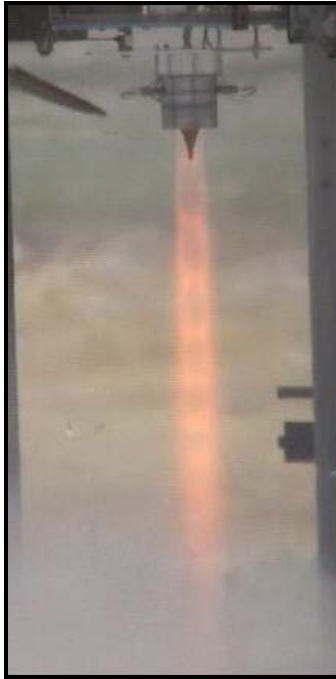
Figure 5. 1000 lbf thrust engine static fire test (06/03)
