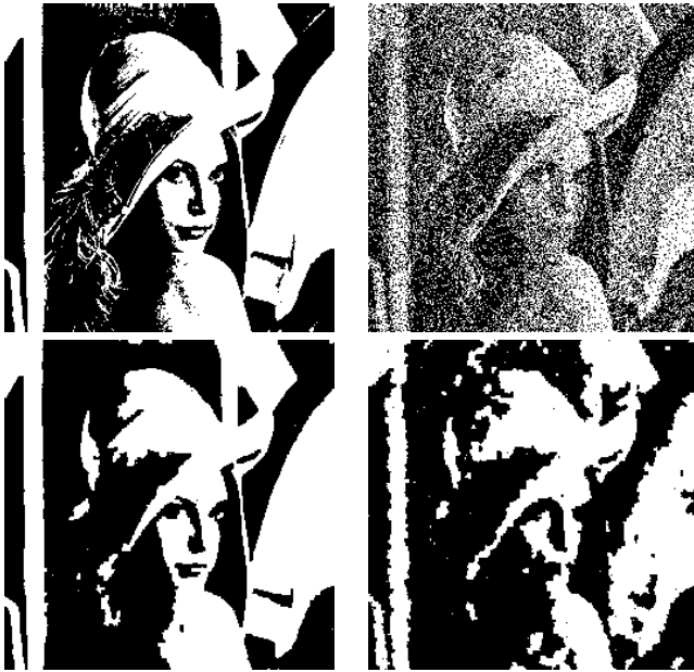
Figure 4: Binary image restoration of Lena via the two-dimensional Ising model. (Upper Left) Original binary image of Lena. (Upper Right) Degraded binary image of Lena ( \sigma^2 = 1 ). (Lower Left) Restored image of Lena using the original binary image of Lena as the external bias field. (Lower Right) Restored image of Lena using the degraded image of Lena as the external bias field.
